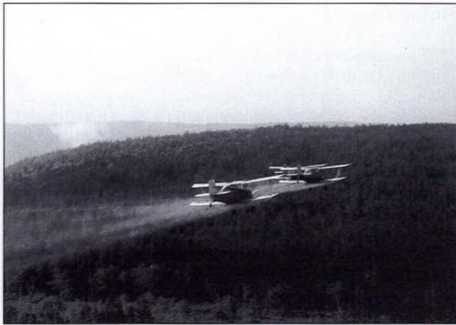
Figure 3. A team of Grumman AgCats spraying Bt on mature red spruce and Norway spruce seedlings planted in a recent strip-cut at Moose River, Cumberland County, Nova Scotia, 1981.
