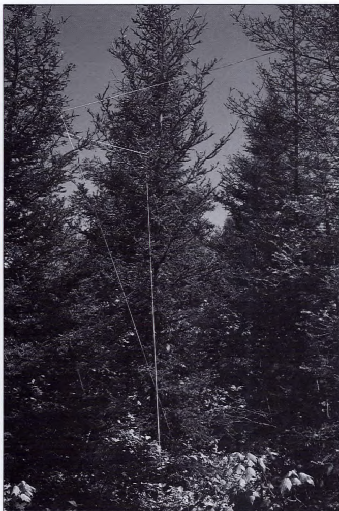
Figure 15. Rope system used to position sentinel budworm egg clusters at different levels in the branch tip area of budworm host trees. The diagonal loops ran between a “pig-tail” stuck in the ground and a ring in the horizontal rope running from tree to tree. These loops allowed the rapid changing of the sentinel clusters. (D. Wallace, Forestry Canada)
