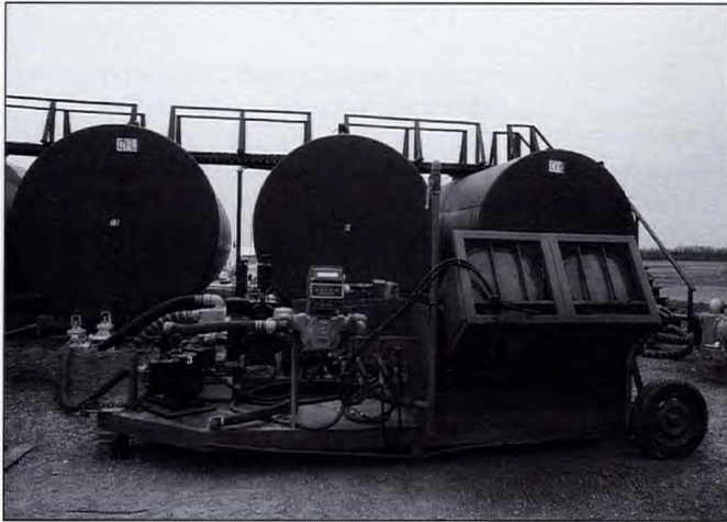
Figure 5. Closed-circuit siphoning of insecticide barrels.
