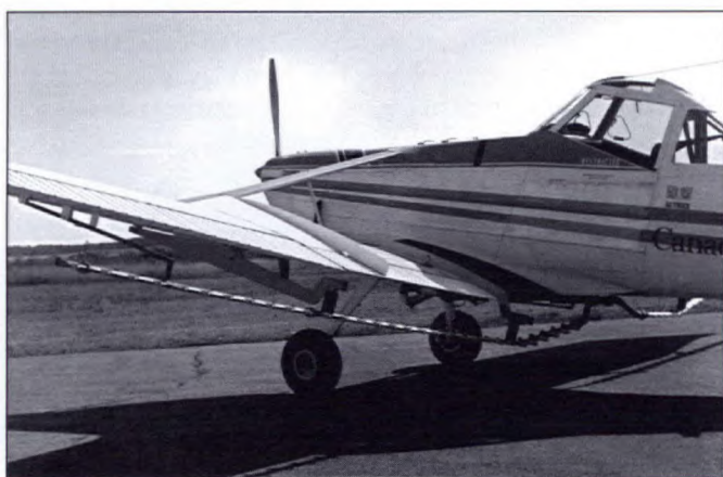
Figure 12. A Thru Valve Boom fitted to a Cessna-188 Ag Truck.
