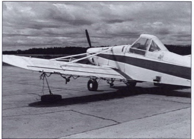
Figure 5. Micronair® AU5000 atomizers fitted to a Piper Pawnee. (M. Pelletier)
