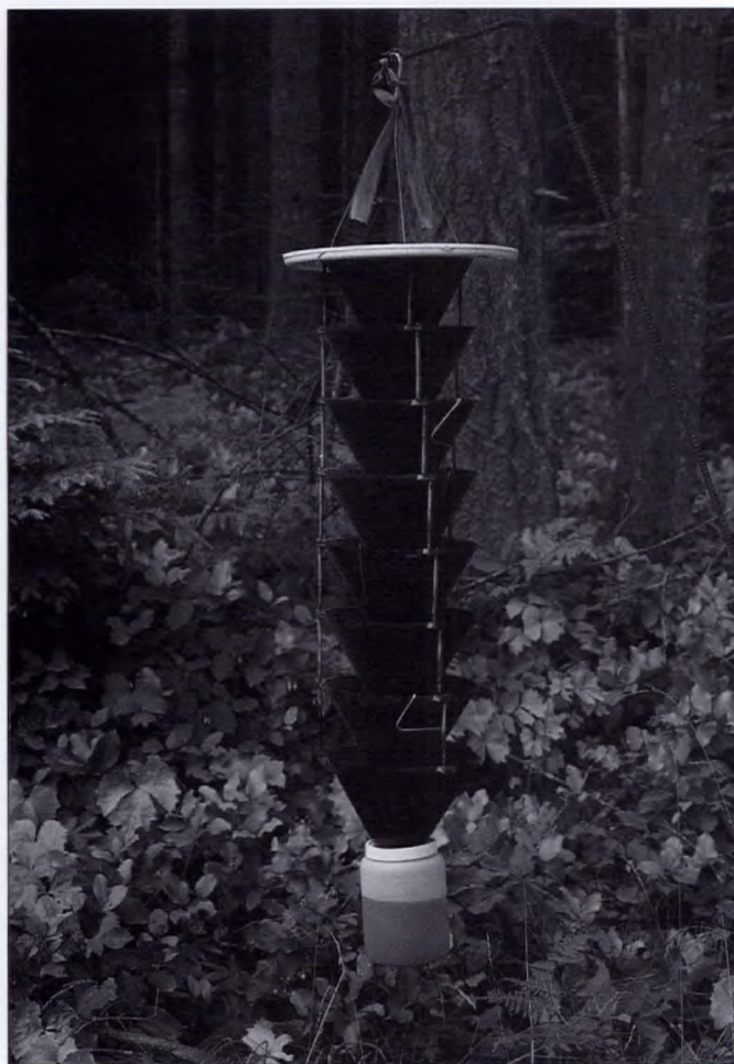
Figure 6. Mass trapping of ambrosia beetles with a Lindgren funnel trap baited with semiochemicals. (H.A. Moeck)
