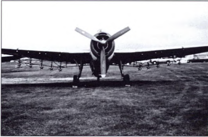
Figure 1. Micronair® AU4000 rotary atomizers fitted to a Grumman Avenger (TBM). (H.J. Irving)
