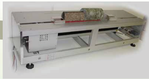
High precision thermal conductivity and diffusivity scanner
