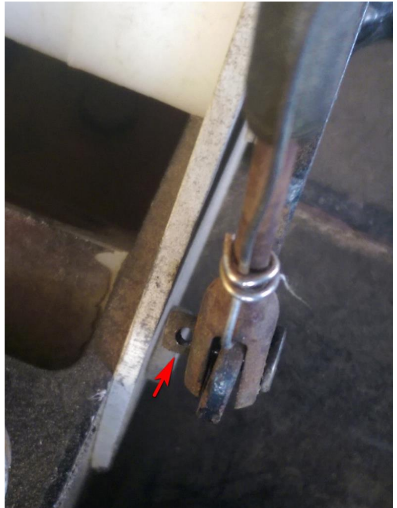
Photo credit: Avery Wagg A missing pin discovered during a pre-flight.
