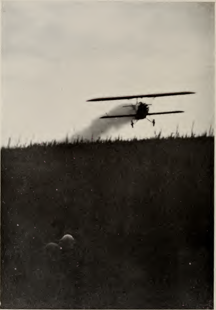
FIG. 19.—Aeroplane sulphur dusting, showing how the dust cloud settles on the crop.
