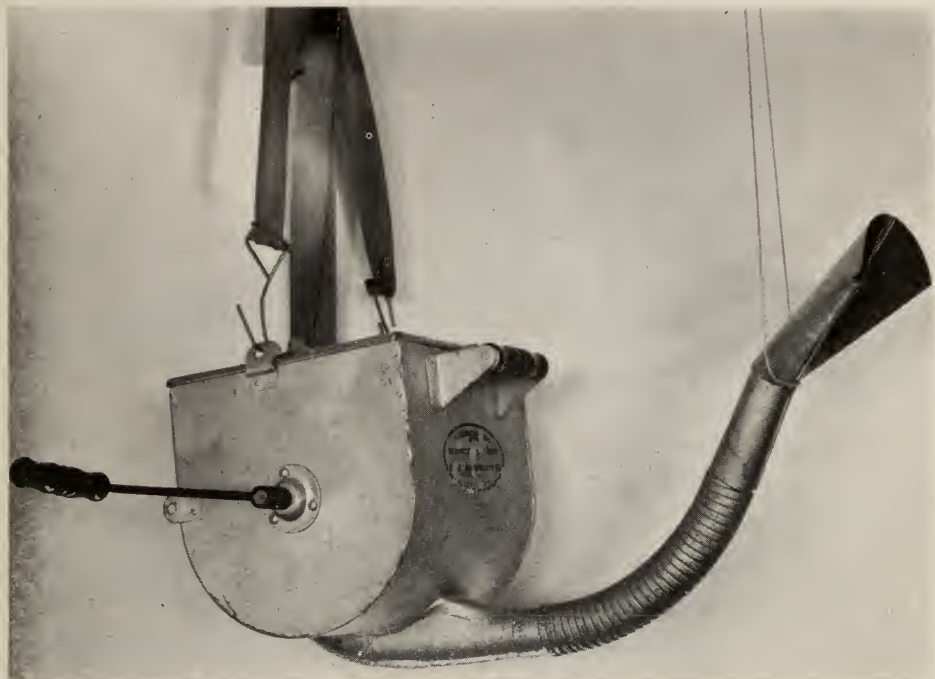
FIG. 20.—Blower dust gun of the type recommended for applying sulphur on small areas for seed or exhibition material.
