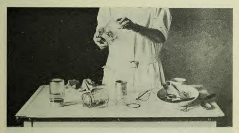
3. Testing Jars Before Sterilizing for Leaks, Cracks, etc.—Put water in jars, adjust rubber, seal tightly, invert and turn on side.
