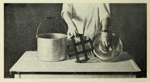
1. Simple Home Canner—Ordinary pot with tightly fitting cover and wooden false bottom to keep jars from breaking.
