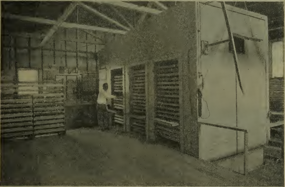
FIG. 3.—View of Penticton cross current, semi-commercial dehydrator with doors removed to give view of drying chamber.
