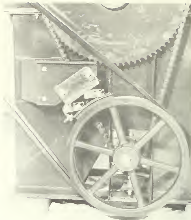
Figure 2.3.14 Anti-reversing brake. Courtesy: Clay Equipment Corp.
