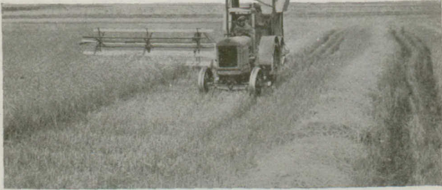
Combine Harvesters, which Reap and Thresh in one Operation, are extensively used in Western Canada
