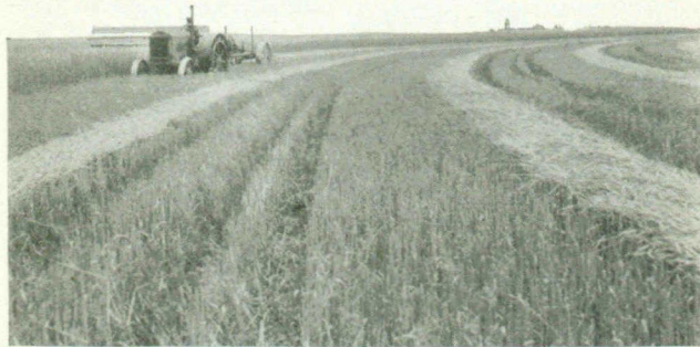
A Swather at work in a Western Canada Wheat Field. The Windrows of Grain are subsequently gathered up and threshed by a Combine Harvester
