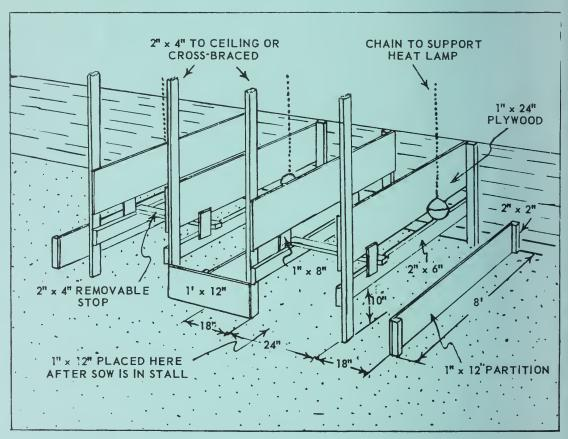
Figure 1 - Detail for construction of two stalls.
