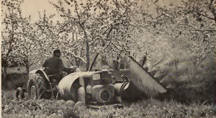
Concentrate sprayer applying dinitro-cresol blossom sprays to apple orchard in full bloom at Summerland.
