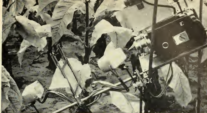
Movie camera used to record flecking (see photo opposite). Flash unit power supply is mounted atop camera and small box behind is operating mechanism. Two flash lamps are used.
