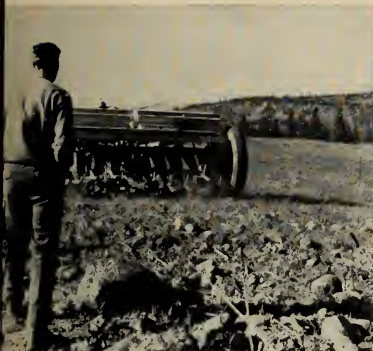
Seeding depleted grasslands with the Oregon Rangeland Drill. Each 20-inch disc is on a pivoted arm and has sufficient weight to carve a furrow even in uncultivated rangeland.
