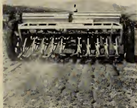
Seeding depleted grasslands with the Oregon Rangeland Drill. Each 20-inch disc is on a pivoted arm and has sufficient weight to carve a furrow even in uncultivated rangeland.
