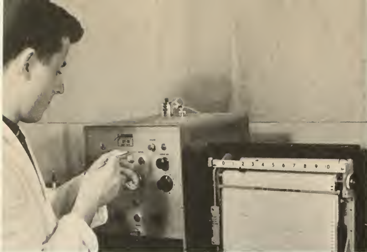
The chemist's gas chromatograph makes possible the accurate determination of pesticides at levels as low as parts per million or trillion.
