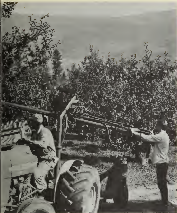
Shake-and-catch harvesting of tree fruits: a hydraulically-controlled boom grasps the tree limb and shakes the fruits on to a canopy from which they are conveyed to a container.
