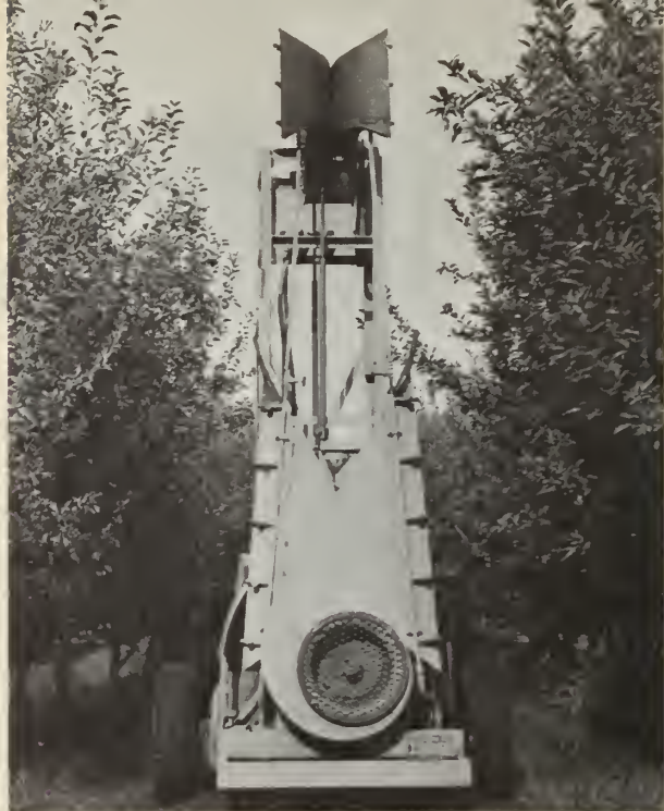
Designed to direct its spray-laden airstream horizontally through 12-foot high trees, this tower-type sprayer built at Summerland Research Station, B.C., uniformly distributes spray material with little loss from drift above the trees. A vertically adjustable hydraulic fan permits spray streams to be matched to tree heights.
