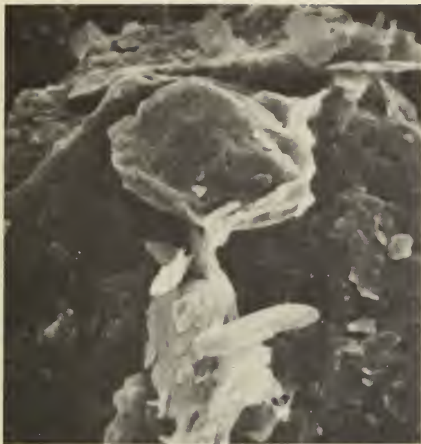
Fig. 1. Clay bridge links two fine silt particles in a fragipan zone of Tormentine soil.
