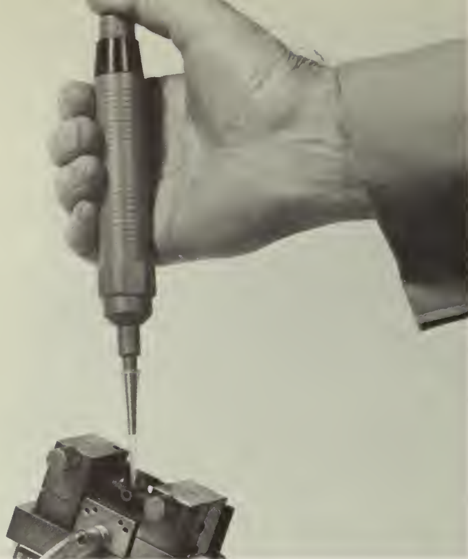
(Above) Introducing a sample solution into the carbon tube by means of a micropipet. (Below) Carbon furnace in operation during the ashing sequence. (Bottom) Furnace at the moment of atomization.
