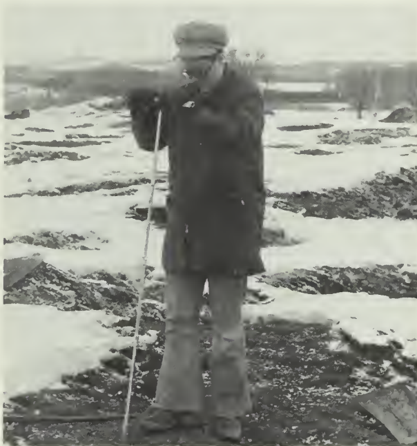
A snow dump at Brandon is sampled for analysis of heavy metal content and salinity of core samples.
