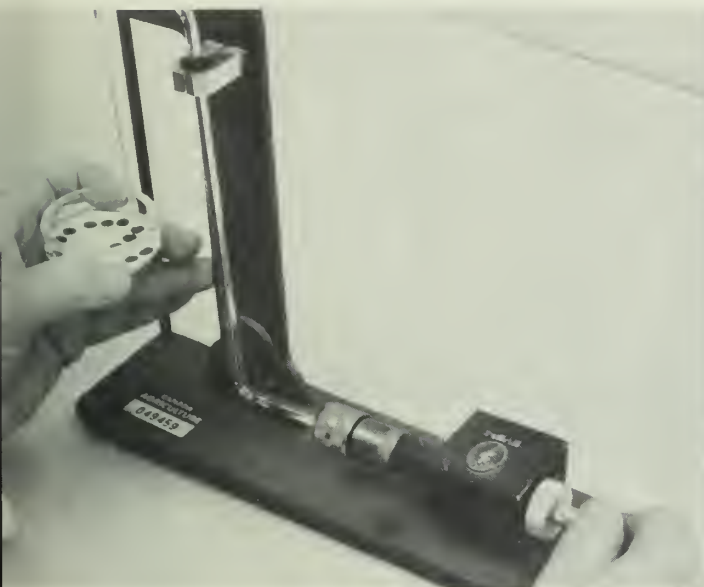
Small amounts of insecticides are applied to discs of lettuce for oral toxicity tests, left, or directly to larvae for contact toxicity tests, right.
