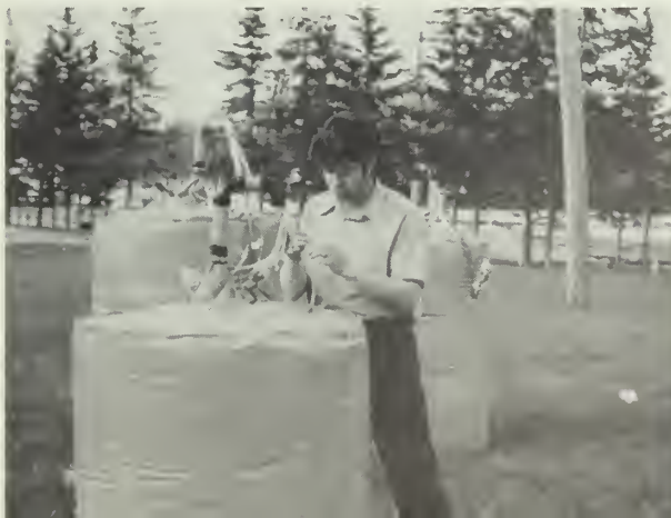
A MERC research assistant takes gas samples in experimental grain bins.
