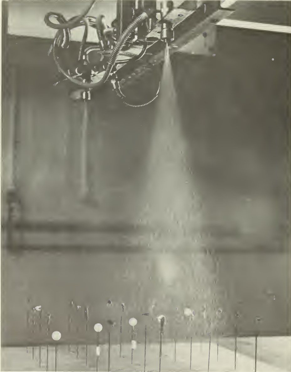
Standard spray nozzles are carried along an overhead track so that sprays can be applied with field equipment under controlled conditions in the laboratory. Half-inch spheres are used as a standard target for comparison in laboratory or field. They have the advantage that they present the same cross-sectional area whatever the direction of the spray. In this experiment deposits are being measured on adult and fourth-instar nymphs in either horizontal or vertical positions.
