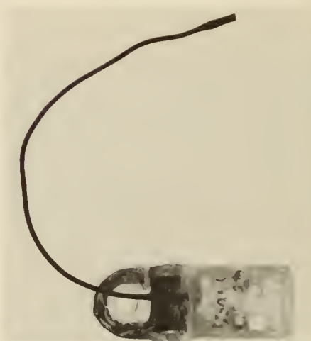
A prototype ear-tag/transmitter used for monitoring brain temperatures in cows. The end of the wire is the sensor that is inserted into the ear canal.
