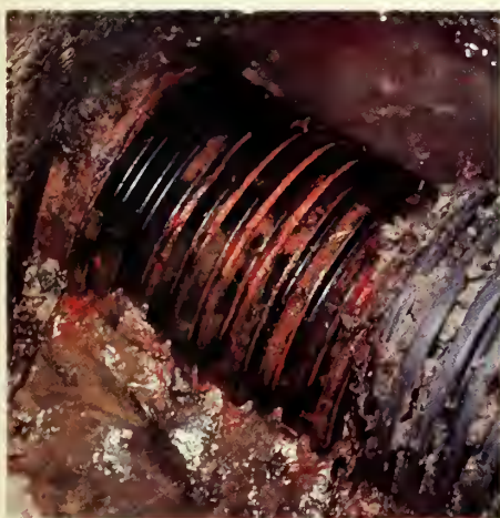
Figure 4. An exposed tile (3 yrs. old) at Aylmer, Ontario, showing the drainage holes being plugged with iron-encrusted bacteria
