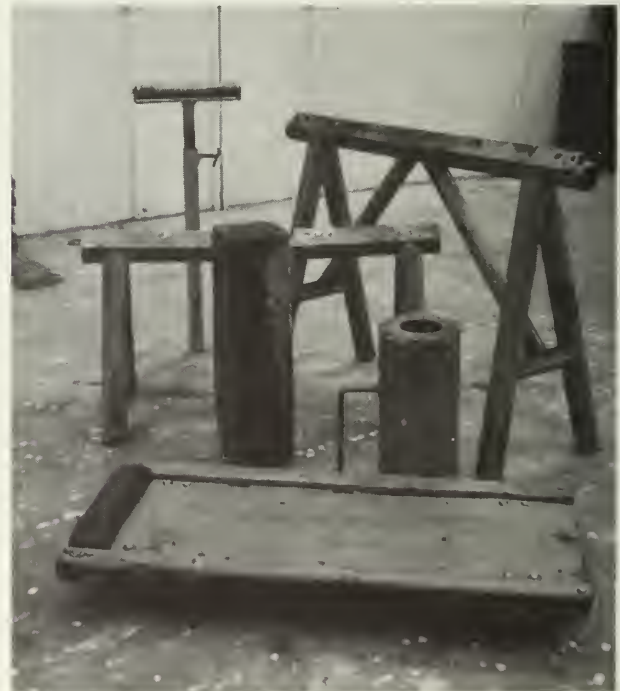
Figure 8 Machine stands made from scrap metal
