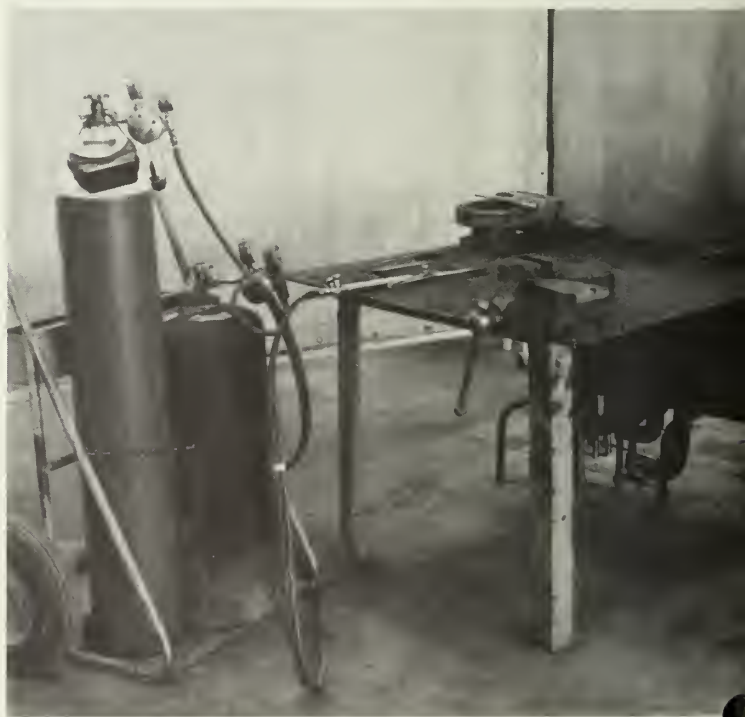
Figure 6 Welding equipment with cart, table and welding screen
