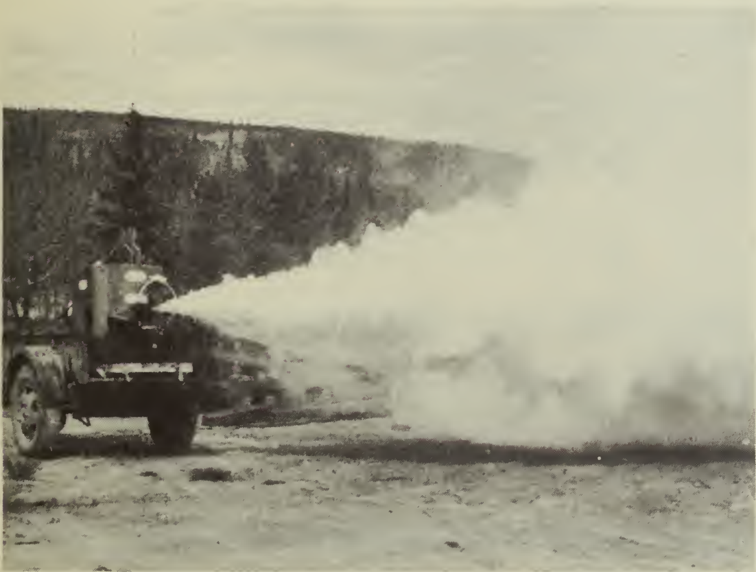
Figure 6. A thermal aerosol generator in operation.
