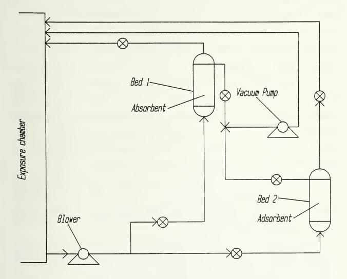
Fig. 10 A schematic diagram of an adsorption pilot plant for handling bromoethane
