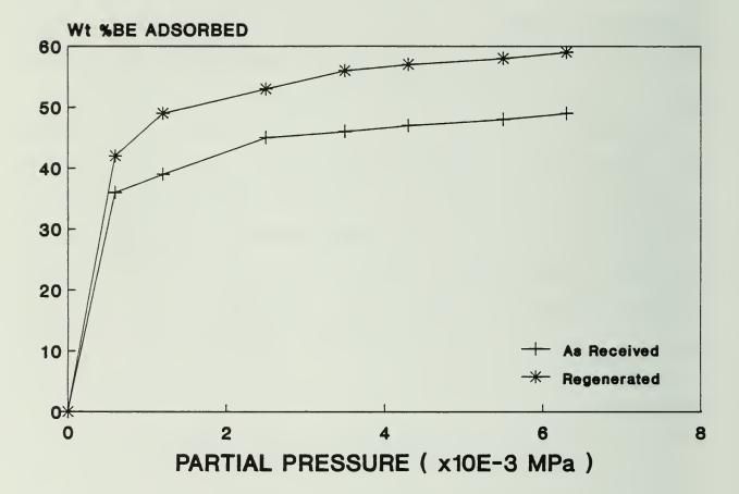
Fig. 3 Adsorption of bromoethane on the "as received" sample of YAO and after regeneration at 150°C
