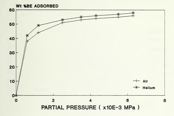
Fig. 5. A comparison of the adsorption equilibria for bromoethane from a mixture of BE-helium and BE-air on YAO at 33°C
