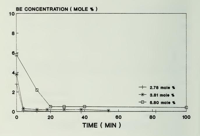
Fig. 9 Bromoethane concentration in the chamber of the benchscale apparatus as a function of time for different initial concentrations of bromoethane in air
