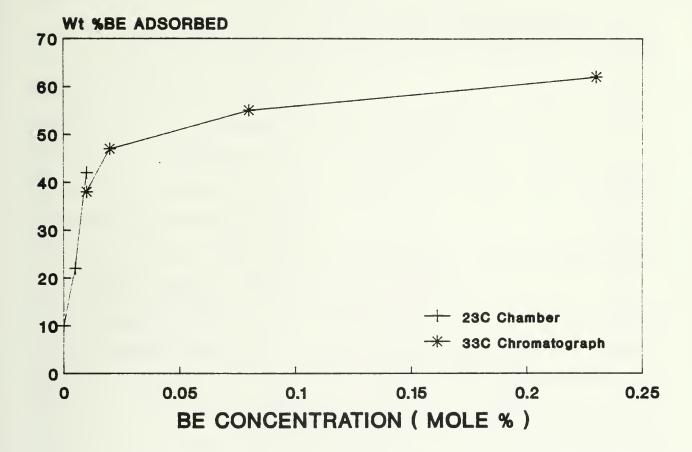
Fig. 8 Adsorption equilibria isotherms for bromoethane on YAO at 23°C determined using the small bench-scale apparatus and at 33°C determined using the screening studies apparatus
