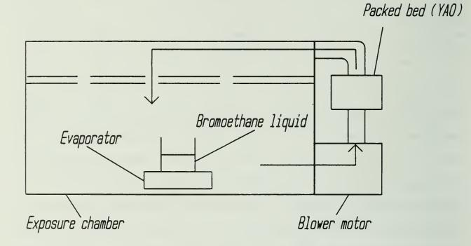
Fig. 7 A schematic representation of the apparatus used for the bench-scale adsorption experiments
