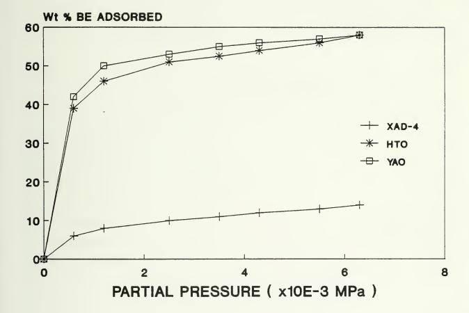
Fig. 2 Adsorption equilibria for bromoethane on YAO, HTO and XAD-4 adsorbents at 33°C
