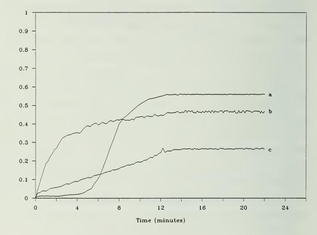
Fig. 6 Breakthrough curves of bromoethane from three mixtures of bromoethane - helium (a), bromoethane - air - water (b) and bromoethane - air (c)
