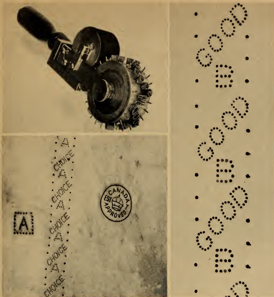
Upper left: Branding roller. Lower left: Carcass showing grader's stamp 'A', choice or 'A' brand mark and Canada Approved stamp. Right: Good or 'B' brand mark.
