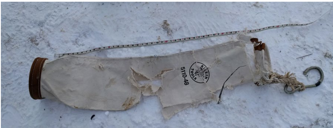
Figure 5. Preform bag at the accident site (Source: TSB)
