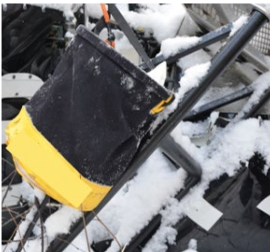
Figure 7. Nose bag attached to the handrail of the Air Stair (Source: TSB)
