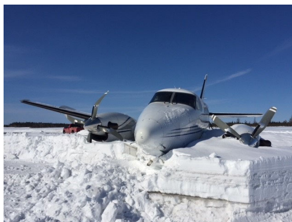
Figure 2. Wreckage of the occurrence Beechcraft King Air A100 (Source: TSB)
