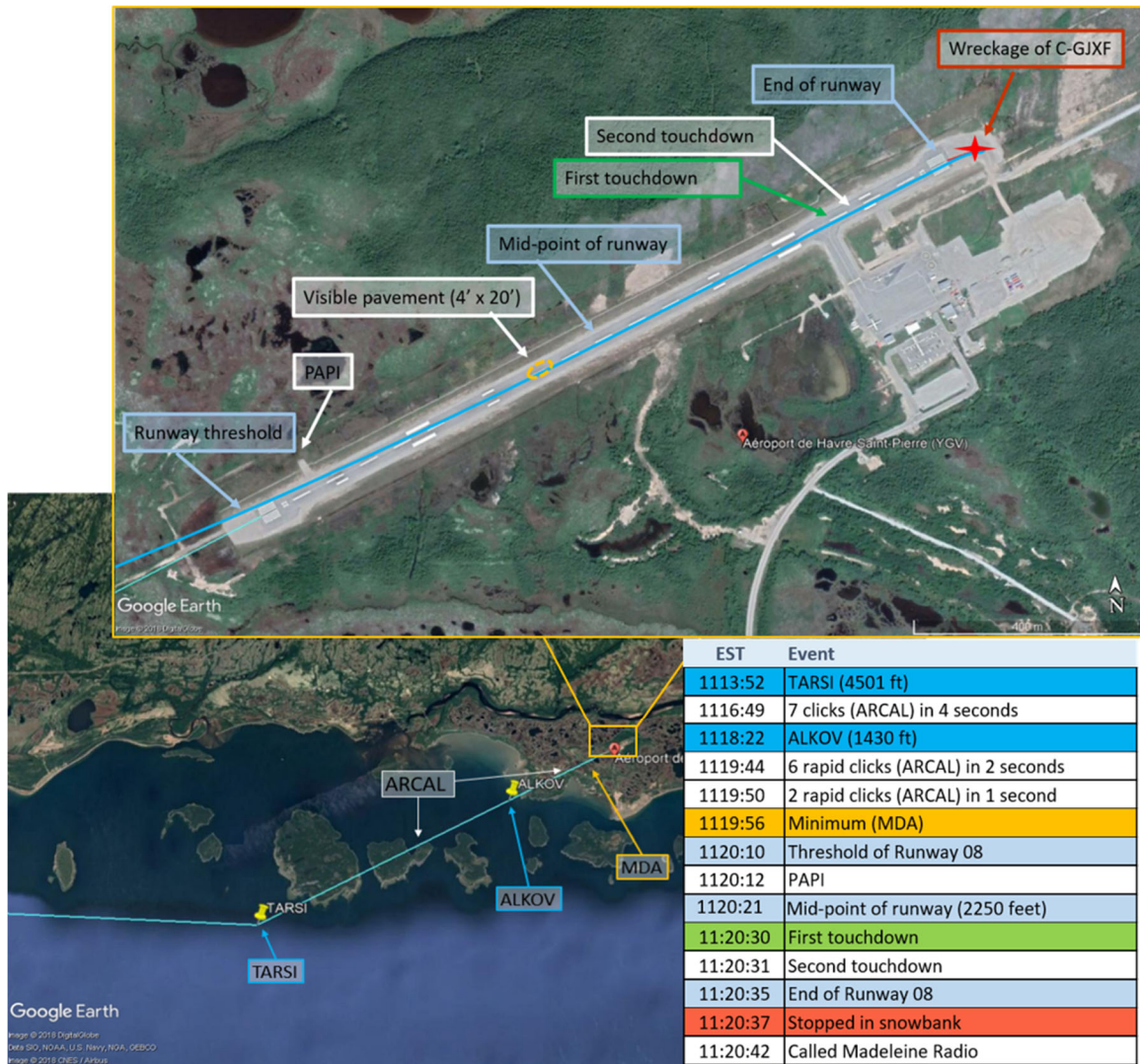
Figure 7. Approach path of the aircraft on final and over the runway (Source: Google Earth, with TSB annotations)
