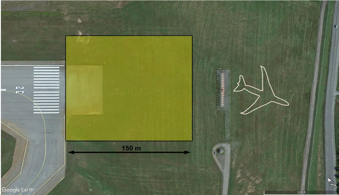
Figure 7. Depiction of Transport Canada's current requirement for runway end safety area on the occurrence runway with the location of the occurrence aircraft after the runway overrun (Source: Google Earth, with TSB annotations)
