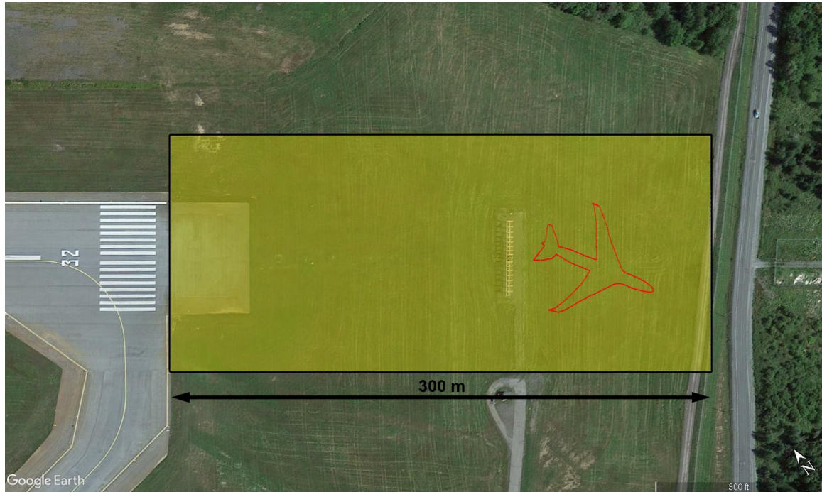
Figure 8. Depiction of International Civil Aviation Organization and TSB recommendation for runway end safety area on the occurrence runway, with the location of the occurrence aircraft after the runway overrun (Source: Google Earth, with TSB annotations)
