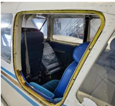
Figure 6. Emergency exit window removed (Source: TSB)
