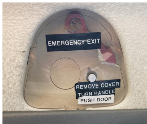
Figure 7. Handle of the emergency exit window with plastic cover (Source: TSB)
