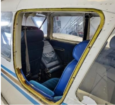
Figure 6. Hublot issue de secours retiré (Source: BST)
