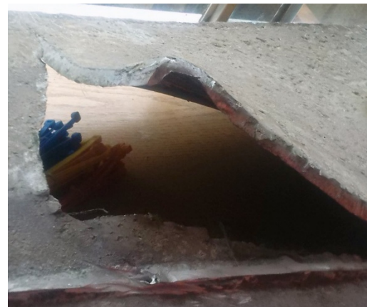
Figure 4. Section of bottom shell plate punctured by rudder (Source: TSB)
