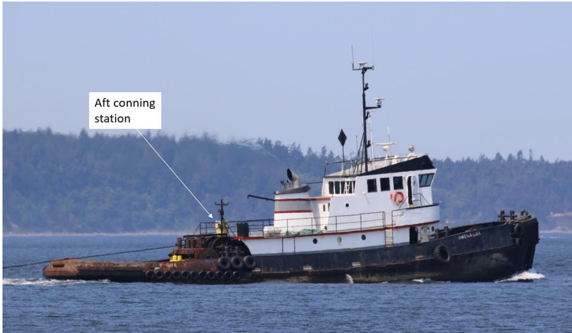
Figure 1. The Mauna Loa , with aft conning station labelled (Source: Jackie Pritchard, with TSB annotations)
