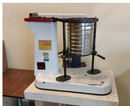
Figure 2 The rotap particle sizing unit used to separate different sized particles of ground oats.
