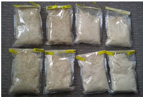
Figure 3 Four bags of whole oats ground with coffee grinders (left) and 4 bags of whole oats ground with rotor beater grinders (right).
