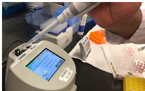
Figure 1 An aliquot of extracted sample being loaded into a lateral flow test strip reader for DON analysis.
