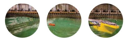
real-world marine conditions. This basin is used to assess the efficiency and safety of marine technologies and evaluate concepts in a controlled environment. Tests performed in this facility include but are not limited to, seakeeping, maneuvering, wave energy conversion, wave impact loads on ships and offshore structures as well as tow out, set down and operation of offshore structures.
