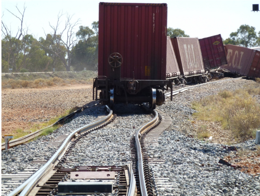
Figure 11 – Track buckling from heat wave, Australia 2013 (Australian Transportation Safety Board)
