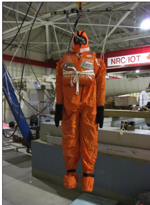
Figure 12: Abandonment Wear 1a worn by a thermal manikin.
