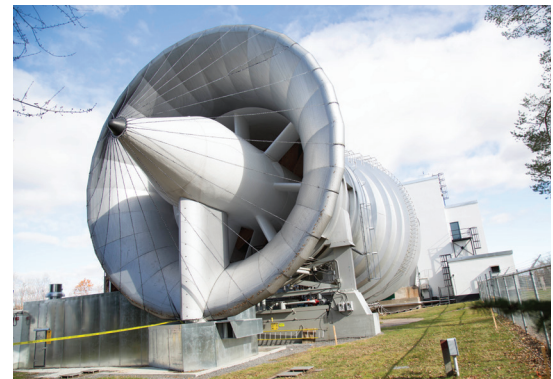
Exterior view of the 3 m x 6 m icing wind tunnel.
