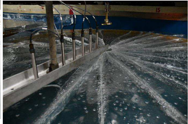
Figure 52: After the test – the indentation event caused the ice to fail mostly via a series of radial cracks.
