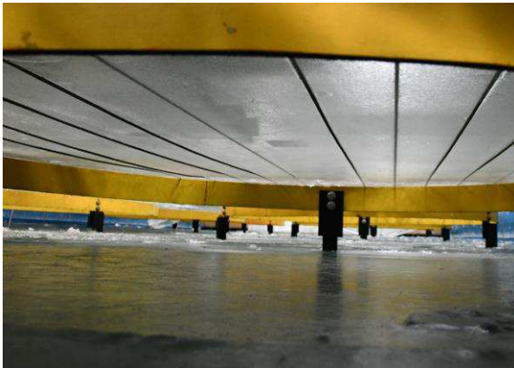
Figure 60: Example (W4) showing cables out of the ice plate at bottom before testing.
