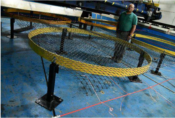
Figure 55: Load frame E2 with the geogrid laid out above it.
