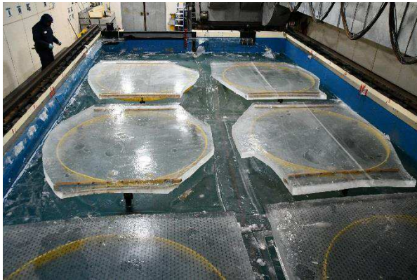
Figure 47: Individual plates after having been cut and the water level having been lowered, bringing them down and allowing them to rest directly on the test frames. Person for scale upper left corner.
