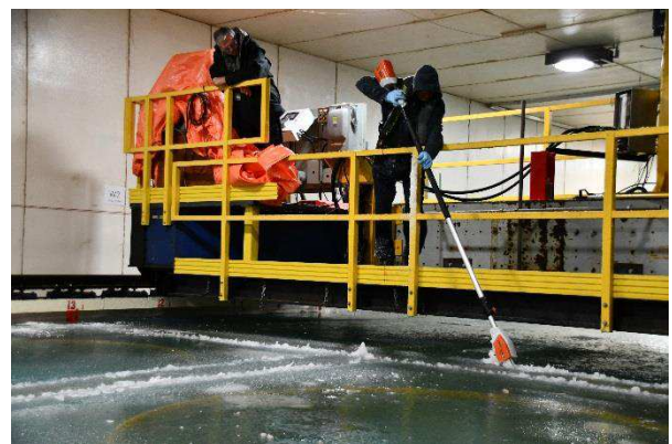
Figure 46: Once the ice above the test frames had achieved target thickness (thereby incorporating the reinforcement), it was cut around each test frame. This was done from the carriage that spans the width of the basin.
