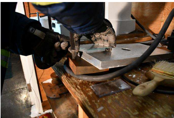
Figure 33: The thickness of the ice slab is reduced by melting it against a plate of aluminum at room temperature (i.e. brought in from outside the cold room). The ice/glass assembly is then returned to the microtome, which is used to further thin the ice (by repeated shaving) to a target thickness of one millimeter.
