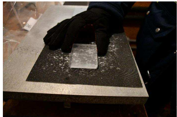
Figure 28: The outcome is an ice slice whose smooth surface is later spot welded onto a clean glass plate with drops of water.
