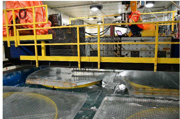
Figure 48: The carriage has been move to the location of a test. Below it is the instrumentation used to monitor the ice loading event and the ice response. Person with orange jacket for scale, upper right.
