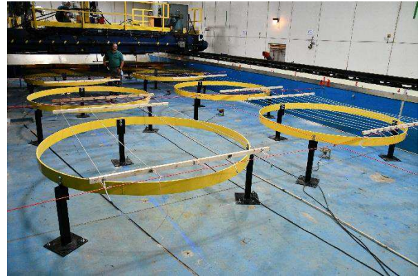
Figure 42: Examples of reinforcement layouts over the test frames. Person for scale again.
