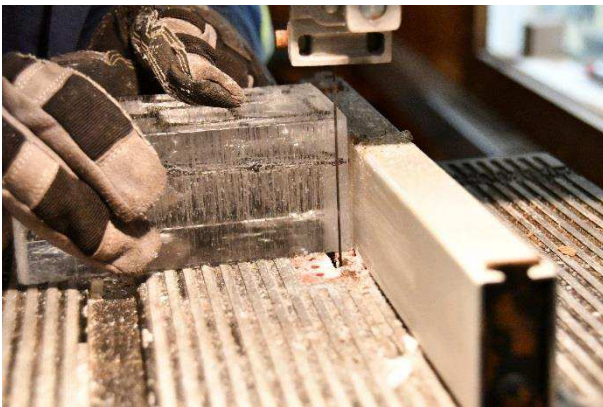
Figure 27: The ice returns to the band saw, and a slice of ice is cut with the smooth surface against the platen.
