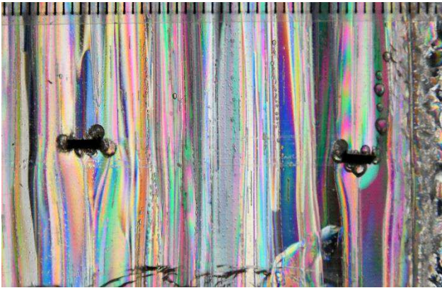
Figure 37: Thin section in cross-polarized light, cut across the membrane. As before, it shows that the crystal are able to grow 'through' the membrane. Scale in millimeter.
