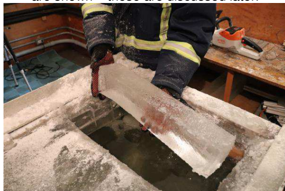
Figure 8: A rough cut beam – this one does not have any reinforcement.
