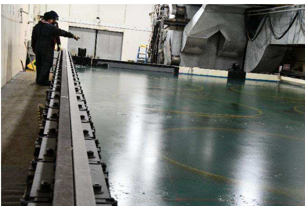
Figure 45: After the seeding event, the water surface is covered with a thin ice layer, which then grows downward (see Figure 9). On the left, next to the two people, is one of the two rails the carriage travels on.
