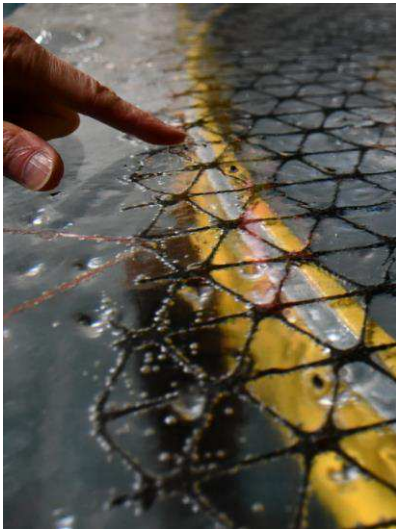
Figure 61: Polypropylene geogrid inside the ice before test E1 – note the presence of air bubbles along the ice-material interface.
