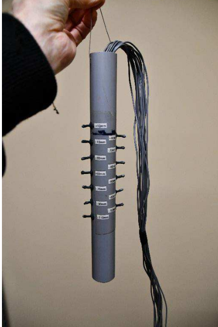
Figure 63: A thermistor profiler was used to keep track of temperature inside and outside the ice.
