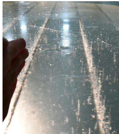
Figure 62: Cables in the ice, also where air entrapment tends to accumulate.
