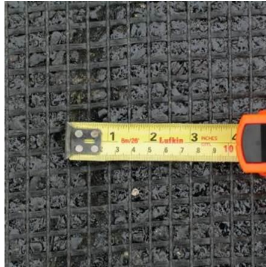
Figure 9: Close-up of a polymer-coated fibre glass 19 .
