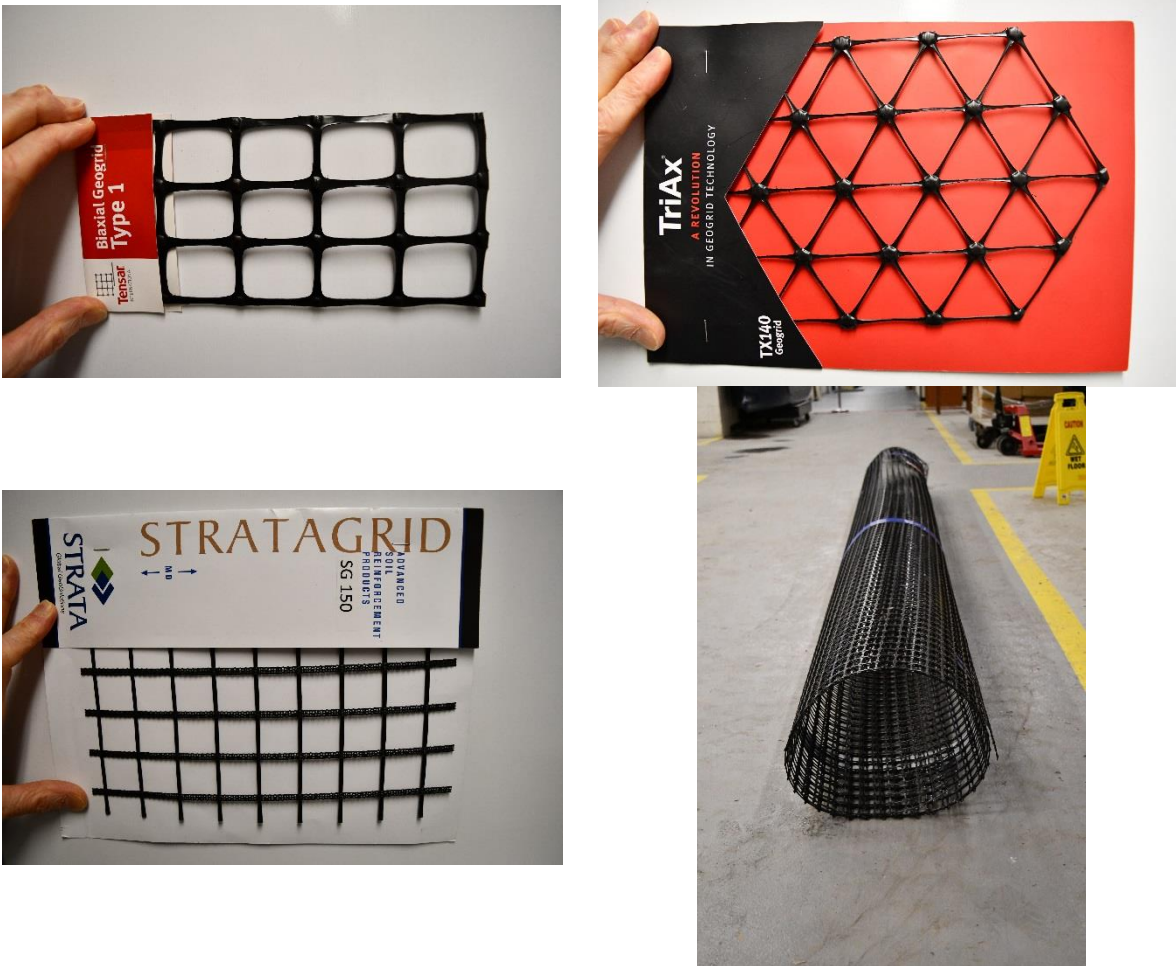
Figure 10: Material selected for testing: Upper left) Tensar’s Biaxial Type 1 Geogrid. Upper right) One of Tensar’s TriAx geogrid. Lower left) Strata’s SG 150. Lower right) A roll of Tensar’s biaxial material.
