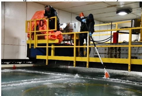
Figure 15: Once the ice above the test frames had achieved target thickness (thereby incorporating the reinforcement), it was cut around each test frame. This was done from the ice tank carriage straddling the ice tank.
