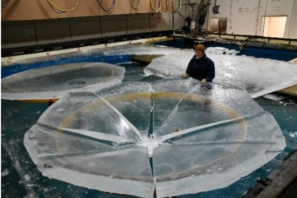
Figure 21: Outcome of a test done with non-reinforced ice. Person for scale.
