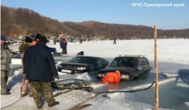
Figure 7: Two of the 20+ vehicles that had been parked on the ice surface before breaking through it. This can be attributed to the time-dependent reaction of the ice cover.
