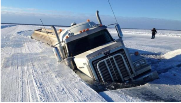
Figure 5: An incident in March 2016 on an ice crossing near Deline, NWT. The circumstances that led to this incident are unknown to the authors. The fracture pattern suggests that pre-existing cracks may have played a role (photo courtesy of NWT Environment and Natural Resources).
