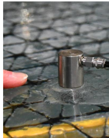
Figure 18: Close-up view of the acoustic sensor, here on ice reinforced with the geogrid.
