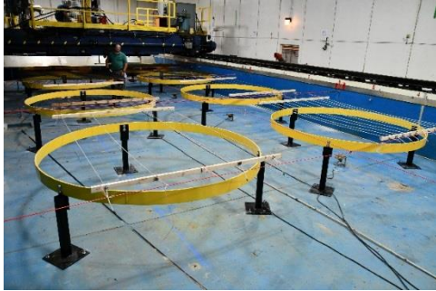
Figure 13: Lay-out of circular frames in the OCRE ice tank, and of the reinforcement above them (person for scale at far end).
