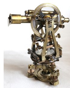
Troughton & Simms theodolite from around 1910, used to measure angles in horizontal and vertical planes — Wikimedia Commons (Colgill, 2020).
