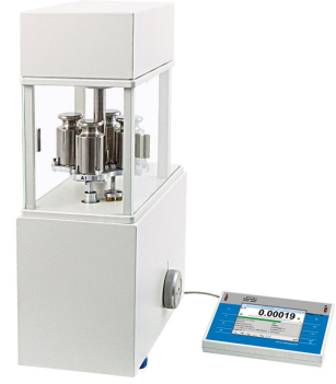
Radwag AK-4/2000 Automatic Mass Comparator (Radom, Poland).
