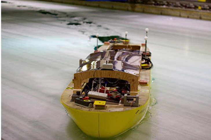
Icebreaker model testing in St-John's.
