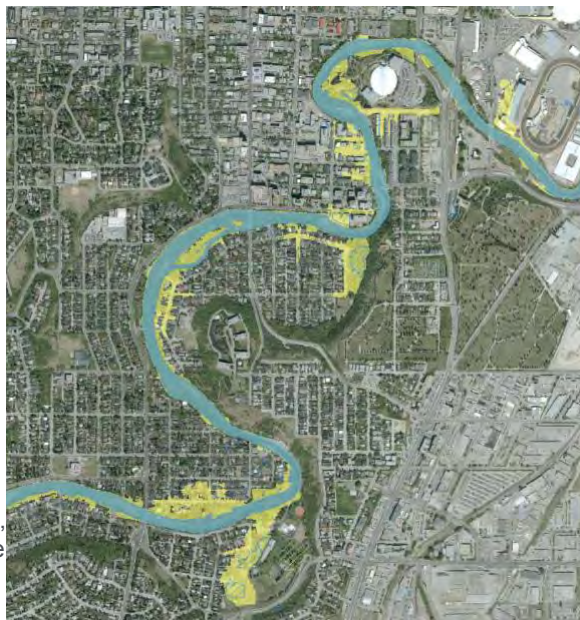
Elbow River 1:20 flood – mitigated to a 1:5 flood (or less), post improvements to Glenmore Dam
