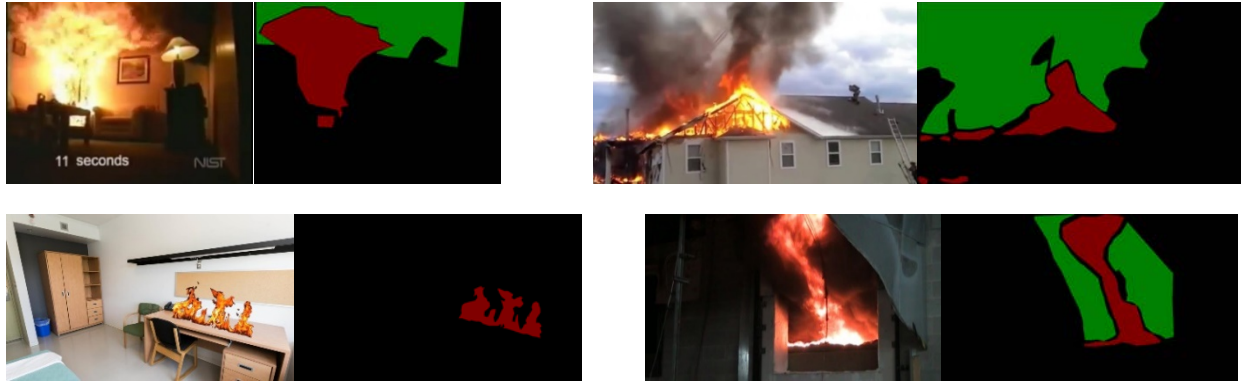
Figure 12: Samples and their annotations (R: flame, G: smoke) from the FS Segmentation dataset. The Upper left image pair is Christmas Tree tests from NIST. The upper right one is image pair from a Fire rescue video posted on YouTube [49]. The lower left image pair is synthetic images generated in this study using Blender. The lower right image pair is from the NRC PRF-07 test.
