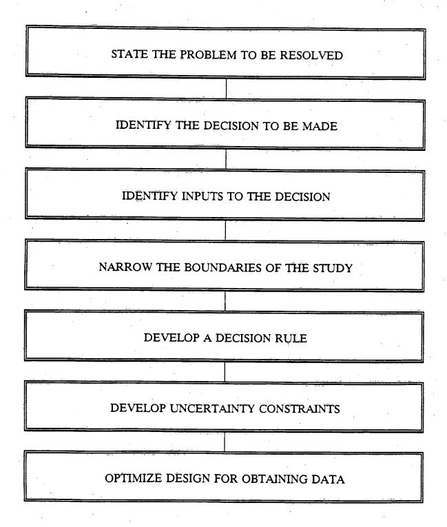
Figure 1. Steps in the Data Quality Objectives Process
