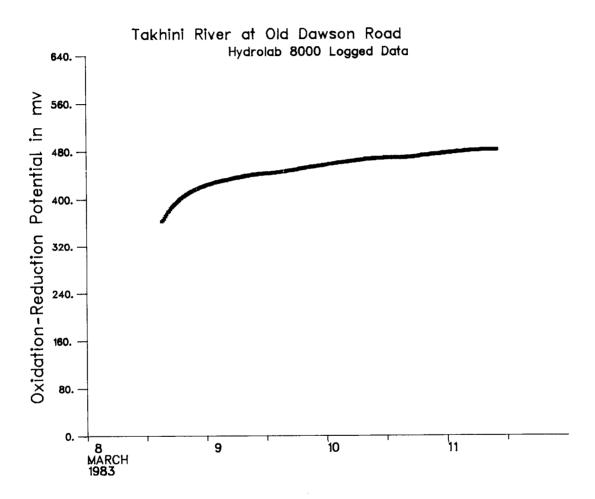
Figure 11 Oxidation-Reduction Potential During March Sampling Period
