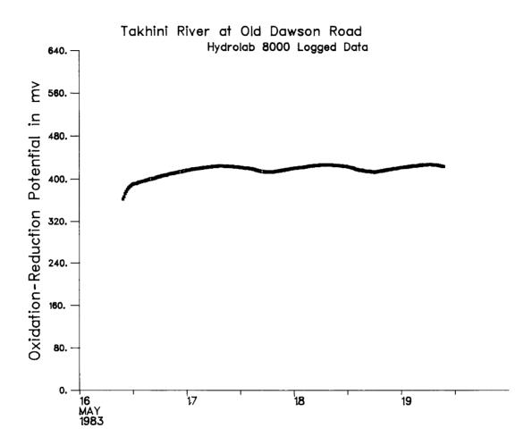
Figure 21 Oxidation-Reduction Potential During May Sampling Period
