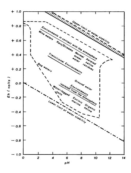
Figure 22 Approximate Positions of Some Natural Environments in Terms of Eh and pH  $\,$
