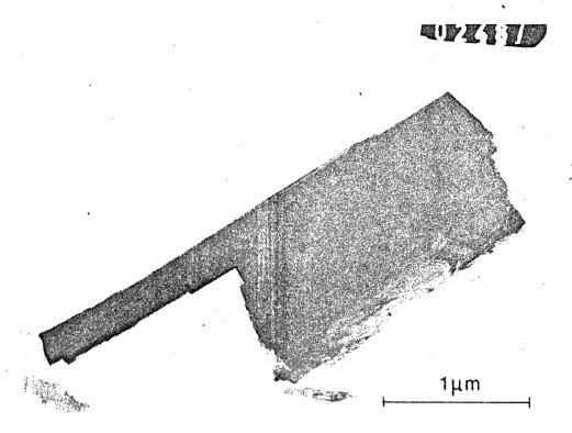
Figure 5. Micrograph and electrondiffraction pattern of fibre in water off Silver Bay.
