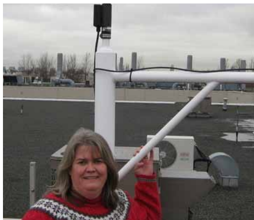
Pat Wong stands with an anemometer, which measures wind, and a snow depth sensor on Environment Canada's Richmond rooftop instrument test platform.
