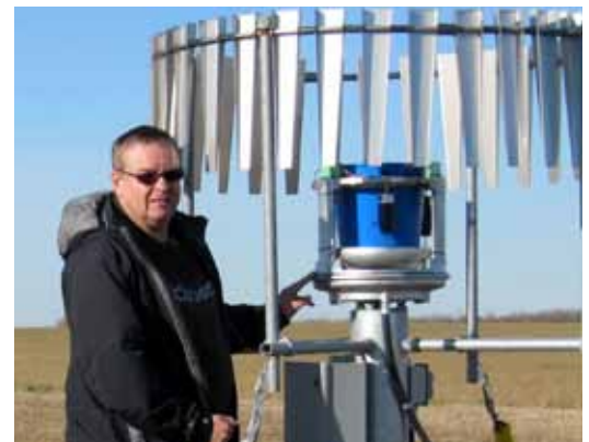
Terry Layes inspects a precipitation gauge that is deployed as part of an automatic observing station in Saskatoon.
