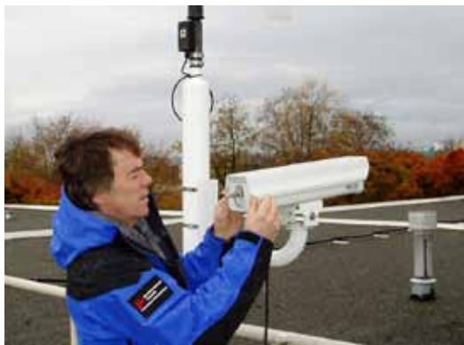
Bill Scott adjusting the alignment of a high-resolution Olympic web-cam in the Meteorological Service of Canada's testing compound in Richmond, B.C.
