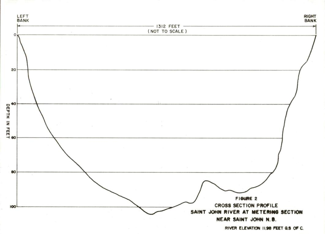
found in the confined channel, had easily accessible banks, and had sufficient velocity at most tidal elevations. The only deficiency was a section of dead water at the left bank and a section of back flow at the right bank. The edge of flow was defined as closely as possible for each measurement.
