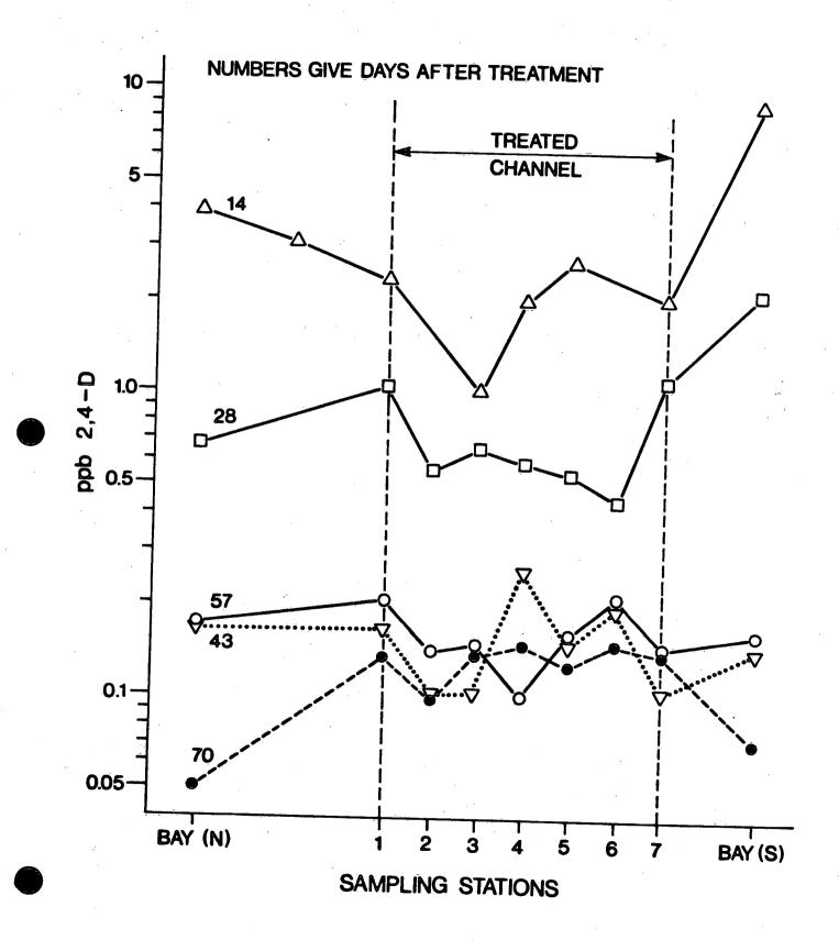
2,4-D in Sediment in Treated Channel.
