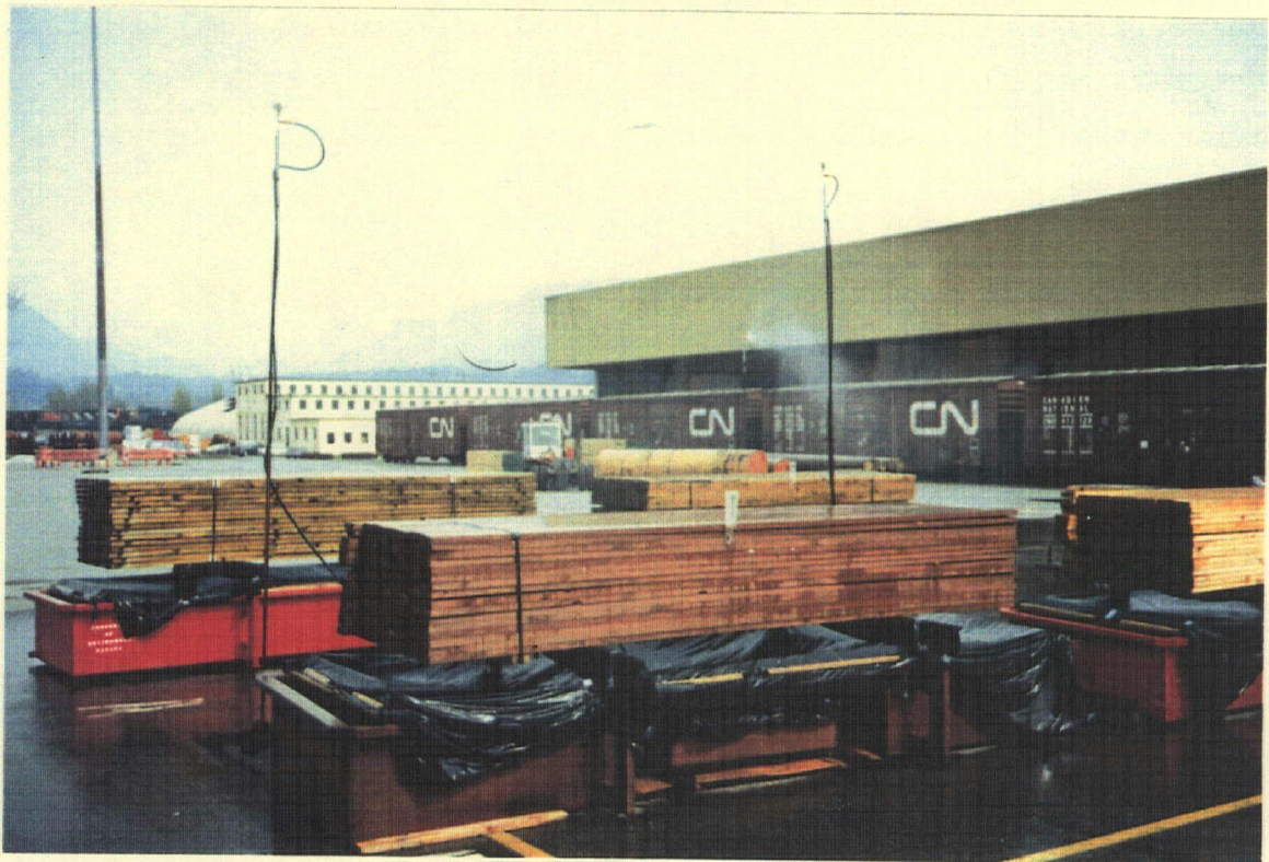
Figure 1. Photographs of the Wood Test Bundles on Leachate Trays on the Lynnterm Site.
