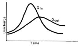
The figure above shows the respective hydrographs and displays the 'storing' effect.
