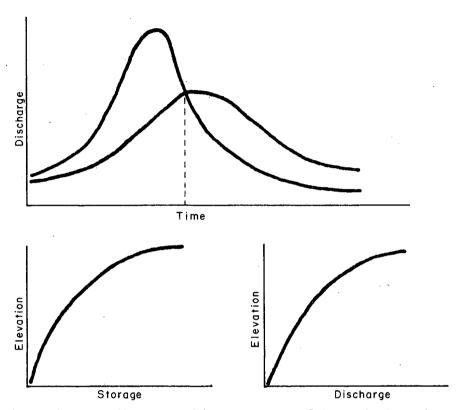
A reach also displays this property of introducing through temporary storage a component to the total flow delay. The secondary component is due to the time required for an inflow to physically traverse the reach.
