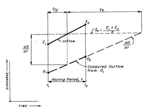
The outflow  $(0_2)$  at the end of the period, for given values of inflow  $(I_m = (I_1 + I_2)/2)$  and outflow  $(0_1)$  at the beginning of the period, is given by
